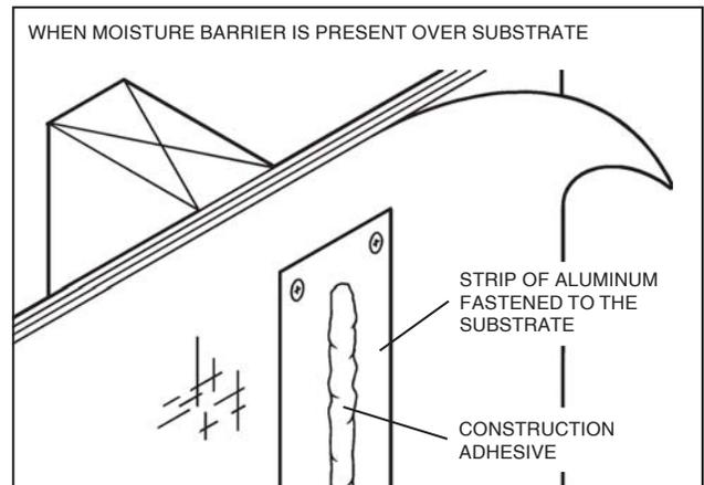
When a moisture barrier is present, a strip of aluminum (approx. 2"-3" wide x 2/3 panel height) must be mechanically fastened to the substrate (**FIG. P**). The adhesive is then applied to the aluminum.
