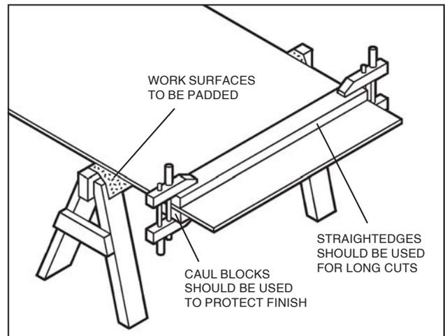
may be clamped to the panel surface. Caul blocks should be used when necessary to protect the painted finish. After cutting, aluminum edges may need filing to remove sharp projections and/or metal burrs (FIG. I) that might prevent the panel from sliding into the molding channel properly. Doing so will also reduce the risk of personal injury.
