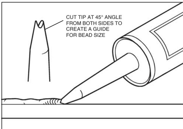
For the two piece system, a continuous bead (a minimum of 1/4" x 1/4") should be placed along the panel edge before snapping the aluminum cover into place (FIG. N).
