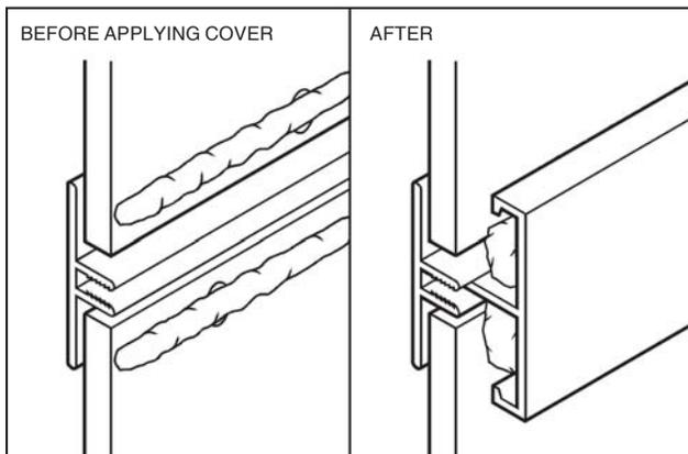
Excess sealant may be cleaned up (FIG. O) after it 'skins over' (approx. 45 minutes) using a non-marring scraper, a clean rag, and mineral spirits (if necessary).
