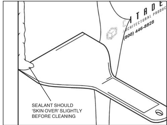
When abutting dissimilar material (i.e. glazing, brick, etc.), allowances must be made for expansion/contraction (minimum 1/4"). Bond breaker tape should be applied to the sheathing prior to the application of the receiver and an approved sealant applied after the panel and aluminum cover are installed (see Typical Details).
